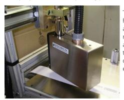
The slide system had to be both accurate and repeatable. In addition, it had to be compact, durable, and cost effective.
