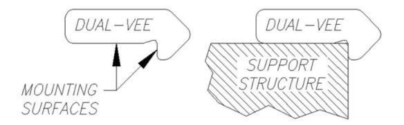
Pay special attention to the track mounting surface because small variations in things like flatness, parallelism and even perpendicularity may result in your wheel not running the way you want it to. Our recommendation is to use a machined register on the support structure (robot frame) in the track mounting locations.
