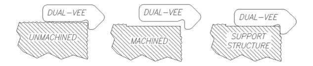
Machining for the track mounting fasteners can also be completed during support member machining. Through hole locations have been standardized on all sizes of DualVee track with dimensions originating from the locating soldier. The catalog dimension "MHL" can be referenced for support structure design.
