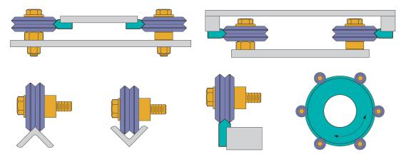
DualVee track is designed with an integrated shoulder and mounting surface. These surfaces are to be utilized when mounting DualVee track to your support structure or in your case, robot frame.
