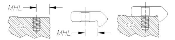
Custom fasteners and hole locations other the ones specified in the catalog "MHL" can be accommodated for a variety of fastening methods. Common DualVee track hole and fastener combinations include clearance holes for screws, through holes with countersinks, and through threads.
